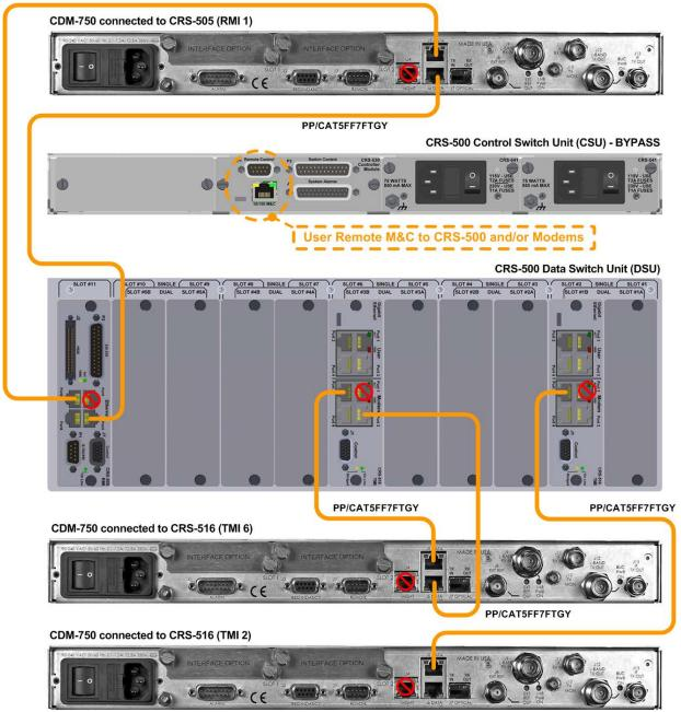
Figure 5-10. CRS-500 → CDM-750/760 10/100/1000 GbE Traffic Data Cabling Example (1:N connections shown for TMs 2 and 6 only)
