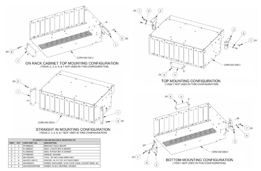
Figure 4-4. CRS-500 Optional DSU Rack Mounting Kit KT-0000072
