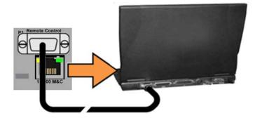
Connect the CAT5 Ethernet cable from the CRS-500 system to an Ethernet port on the User PC via a hub or a switch, or direct connection. Note that the location for this M&C connection depends both on the deployed modem model and the mode of Ethernet in use. See Chapter 5. CABLES AND CONNECTIONS for details.
