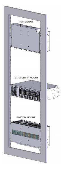
Figure 4-3. CRS-500 DSU In-Rack Mounting Examples (Uses Optional CEFD Kit KT-0000072)
