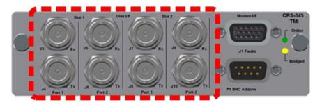
The CRS-345 TMI BNC connectors group provides a multiport Unbalanced G.703 User Data Interface.
