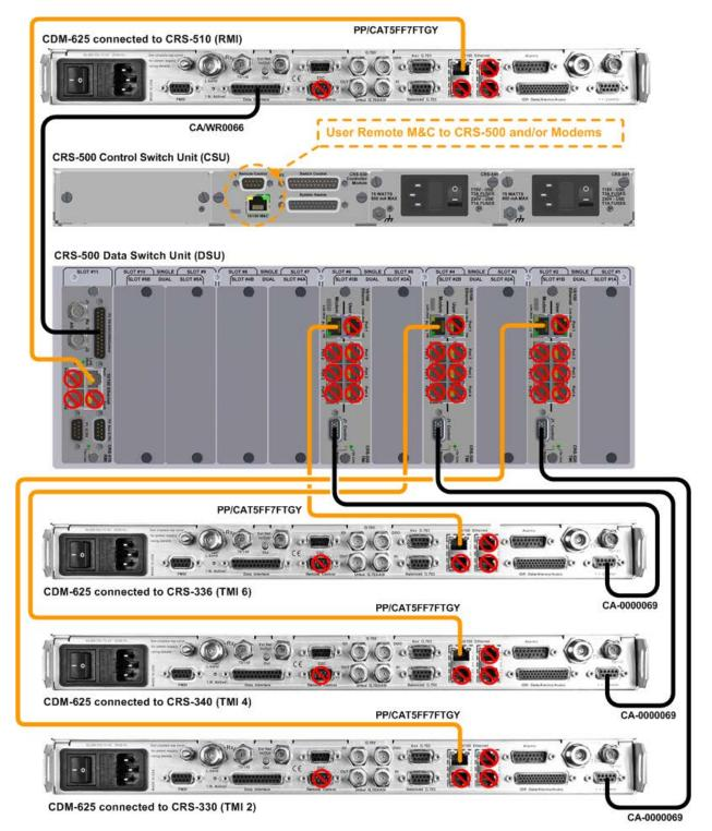
Figure 5-4. CRS-500 → CDM-625/625A Control & Ethernet System Comm Cabling Example (1:N connections shown for TMs 2, 4, and 6 only)
