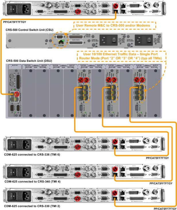
Figure 5-5. CRS-500 → CDM-625/625A 10/100 Ethernet Traffic Data Cabling Example (Single Port Router Mode, 1:N connections shown for TMs 2, 4, and 6 only)
