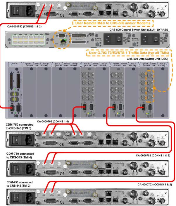
Figure 5-11. CRS-500 → CDM-750/760 G.703 Unbalanced Traffic Data Cabling Example (1:N connections shown for TMs 2, 4, and 6 only)
