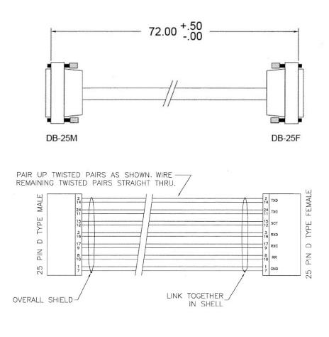
Figure A-4. RMI Control Cable (CEFD P/N CA/WR0066)
