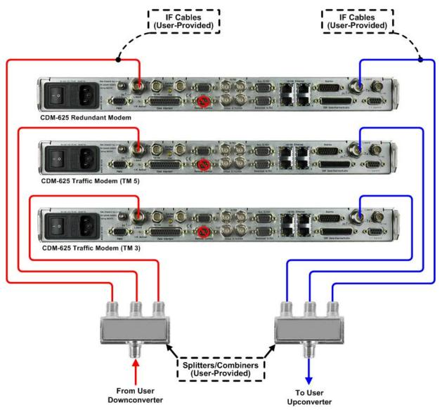
Figure 5-12. CRS-500 1:N IF Cabling Example 1 – Single Transponder Configuration (No ISU) (Connections shown for TMs 3 and 5 and 8 only)
