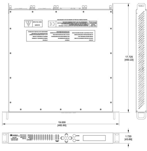
Figure 2-1. CRS-500 CSU Dimensional Envelope
