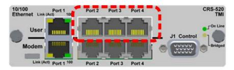
The CRS-520 TMI provides four standard RJ-45F User Interface ports, operating at 10/100 Mbps, half and full duplex, auto-negotiating for Ethernet Router Modes.
