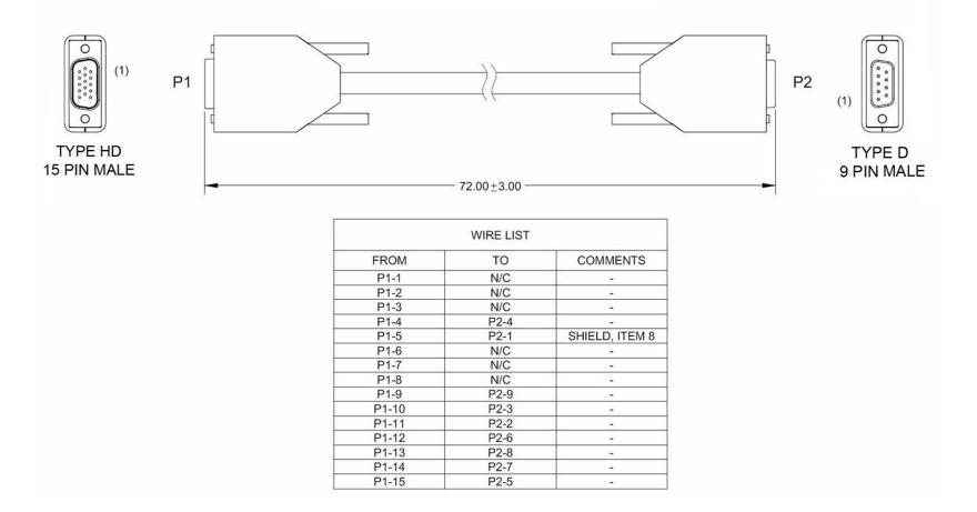
Figure A-5. CDM-625/A, CDM-750/760 Control Cable (CEFD P/N CA-0000069)
