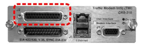
This 25-pin Type 'D' female connector provides the **EIA-232/422/V.35** User Data Interface on the CRS-316 TMI.
