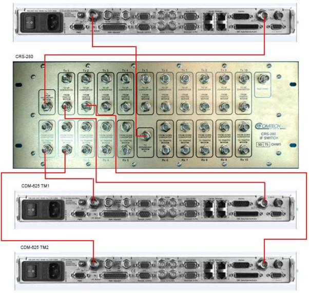
Figure 5-13. CRS-500 1:N IF Cabling Example 2 – CRS-280 → CDM-625/A (Connections shown for TMs 1 and 2 only)
